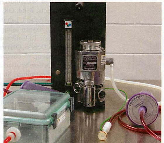
FIGURE 2 | Passive scavenging equipment. Activated charcoal canisters connected to the induction chamber (left) and to the discharge tubing of the non-rebreathing facemask (right) provided passive scavenging of WAG during anesthesia induction and maintenance, respectively, in Condition 1 and Condition 2.
